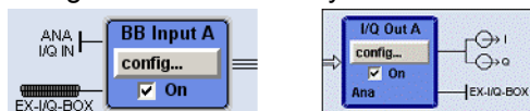
Fig. 6-16: Indication of an R&S EX-IQ-BOX in a generator block diagram at the example of the R&S AMU200A
