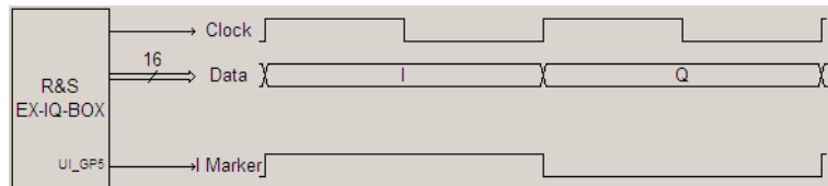
Fig. 7-14: User defined > Signal flow: I/Q OUT parallel, single data rate, I/Q inter-leaved
